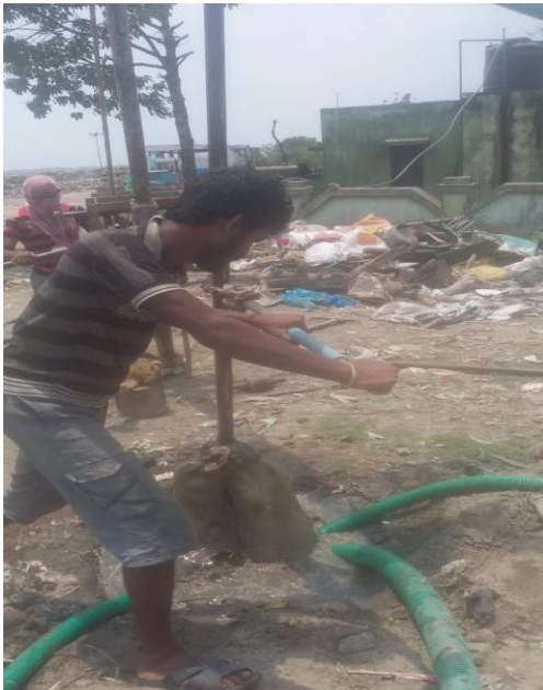
Figure 5 Soil sampling for Geotechnical and Topographical Survey at Mollar Bheri
